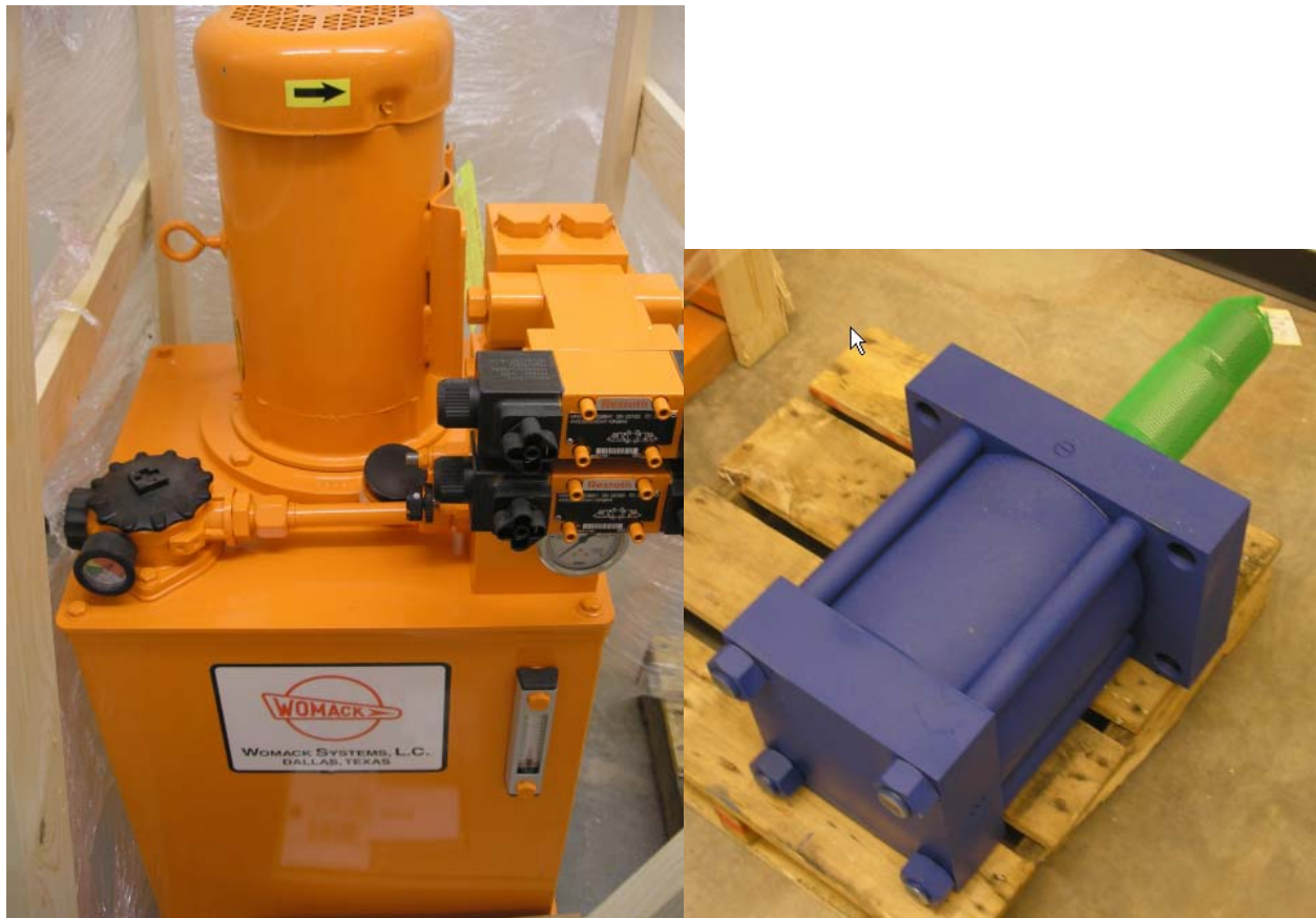
Figure 3. Pictures of the hydraulic power unit and the 8-in bore cylinder
